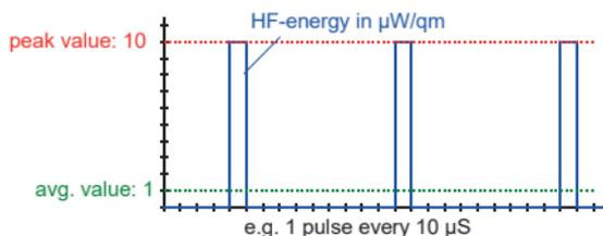
With the switch set to "Peak", the meter will display the full power flux density of the pulse (10 μW/m<sup>2</sup> in the graph). With the switch set to "RMS", the meter will take the mean of the power flux density over the total period of time, for instance 1 μW/m<sup>2</sup> in the above graph (= ((1 x 10) + (9 x 0)) / 10).
