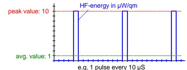
Note: The **peak HF radiation value**, not the average value, is regarded as the measurement of critical "biological effects". The peak value is displayed in the switch setting: "Peak". The average value is displayed in the switch setting: "RMS".
